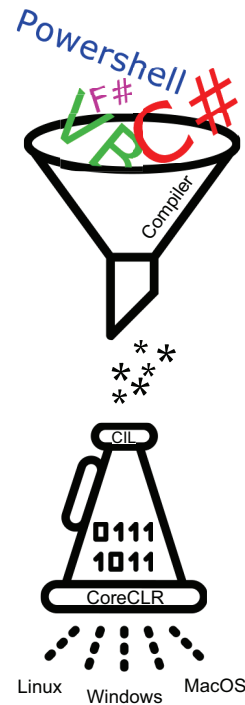
Figure 2.7 CoreCLR can JIT-compile for targets such as Linux, Windows, and macOS. This allows for cross-platform execution of C# code.
