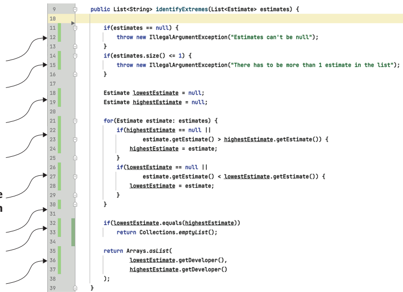
Figure 1.3 The result of the code coverage analysis done by my IDE, IntelliJ. All lines are covered.
