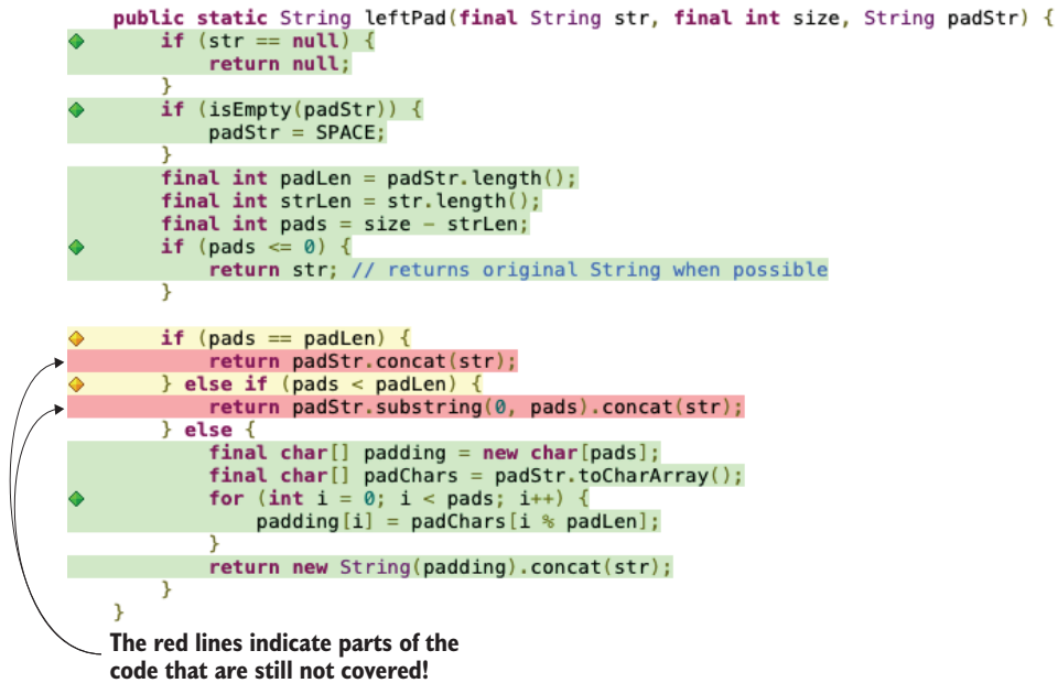
Figure 3.8 Code coverage achieved by the specification-based tests for the leftPad method. The two return lines near the arrow are not covered; the if and else if , also near the arrow, are only partially covered. The remaining lines are fully covered.
