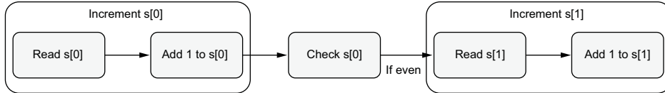
Figure 12.15 Three main steps: increment, check, increment
