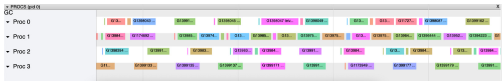
Figure 12.41 About 50% of CPU time is spent handling goroutine switches.
