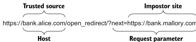
Figure 13.5 URL anatomy of an open redirect attack
